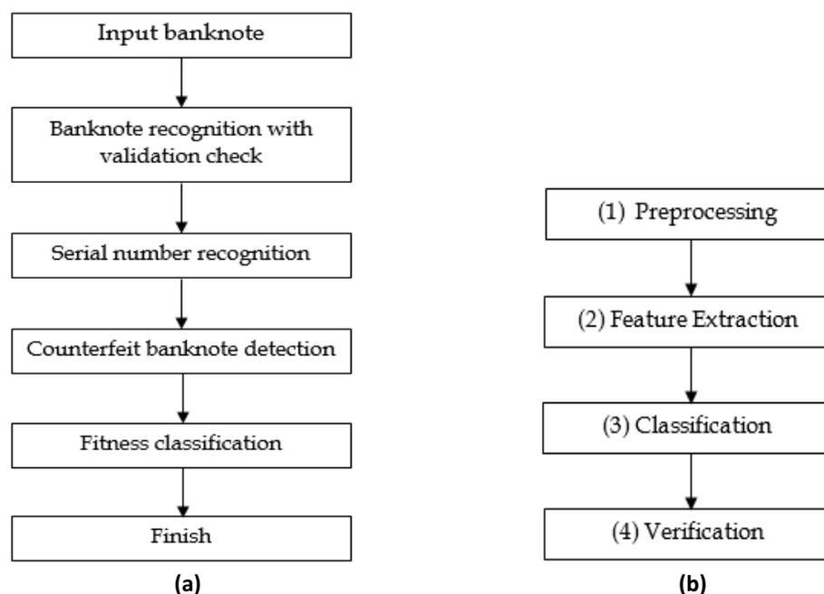
Fig. 1. a) Elaborate banknote recognition process flow in an automated device; b) Modest banknote recognition process flow.
